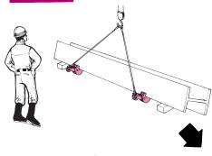
For Model AC clamp, there is an angle where the clamping force may not be sufficient, depending on the direction of a lifting load. When using, attention must be paid to the direction in which the load is being pulled or lifted.
